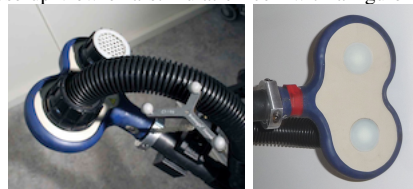
Fig. 1. Close-up view of a stimulation coil with a figure-of-eight shape.
