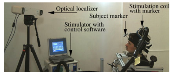
Fig. 2. TMS setup with localizer for navigation.
